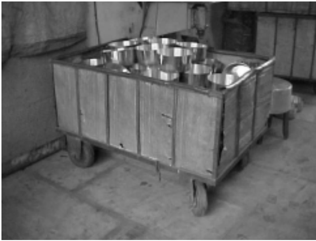
Figure 3. Improvements in a small metalworking factory in Vietnam, resulting from a WISE training course. Roller conveyor to carry heavy materials with a guard on rotating parts of the machine (3a). Wheeled container to carry their products (3b).
