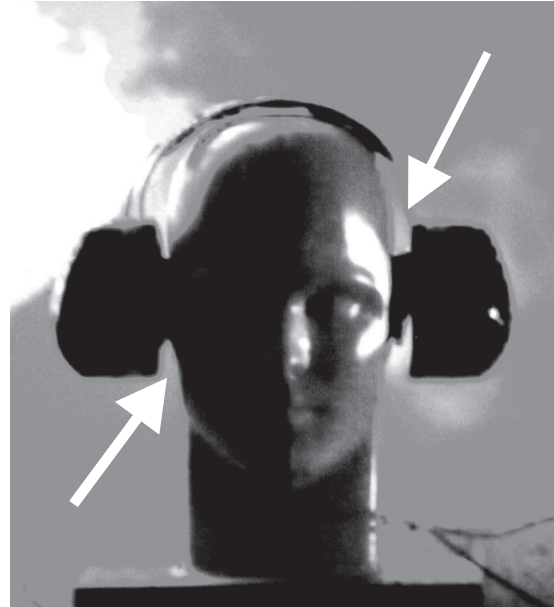
Figure 10. Ear muff on an artificial head exposed to a shock wave with a 190 dB peak pressure level.
