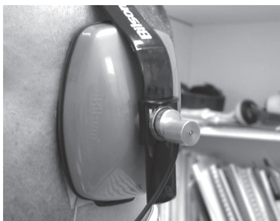
Figure 1. The mounting of the microphones.
