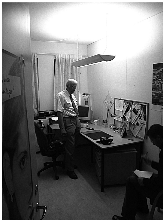
Figure 1. Typical VDU screen placement for a single-occupancy office—in the corner of the table close to the window. Notes. The luminaire had 3 \times 36 \text{ W} lighting tubes; one was lit downwards, two were lit upwards giving luminance from the ceiling of 380\text{--}450 \text{ cd/m}^2 .
